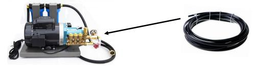
3) Run the nylon to the vertical blank mist section. Or continue using the nylon to the application.
